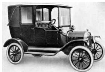
The original brass radiator was replaced by a larger black one in late 1916. 'Improved' cars from 1925 featured nickel-plated radiators.
